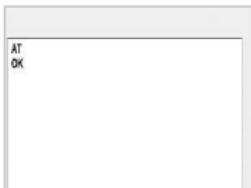
4. In the hyper-terminal Connection window Type AT and Press Enter OK response you get ready to Use Modem.
